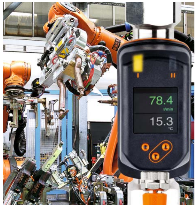
Monitoring the cooling circuits at a welding gun
